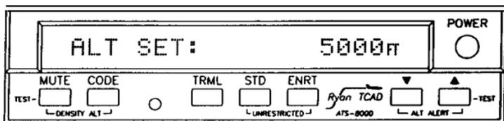
The ▼ and ▲ buttons can be used separately to adjust the displayed altitude to an assigned or desired altitude (or flight level). If no button presses occur for 8 seconds, the Altitude Alert is engaged at the displayed altitude, and TCAD will return to the collision avoidance display. If desired, the Altitude Alert can be manually engaged by pressing the ▼ and ▲ buttons simultaneously while the ALT SET: message is displayed.
