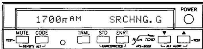
This illustration shows TCAD has automatically entered the Ground Mode, and is operating in the Search Configuration. All tones are muted (hence the "M") and aircraft at and below 100 feet above the host encoded altitude are not displayed (see Section III for more on Ground Mode).
