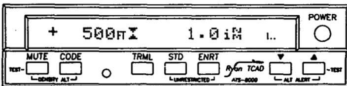
Passing through 2,900 feet, traffic monitored by the TCAD nears the Air Traffic Shield. As shield penetration is detected, a tone sounds. The traffic shows 500 feet above the host aircraft, closing in altitude, 1.0 iNM. The iNM is getting smaller, indicating closure in range. The traffic is acquired visually, crossing from left to right, descending. Climb is momentarily slowed to allow the traffic to pass well clear.
