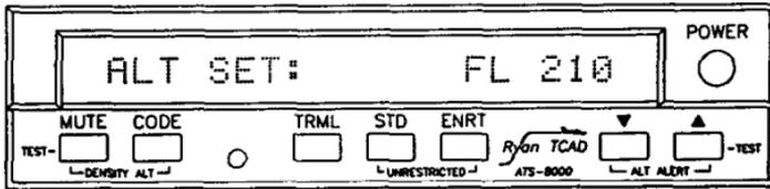
Cleared out of 4,000 feet for Flight Level 210. Reset the Altitude Alert to FL 210.
