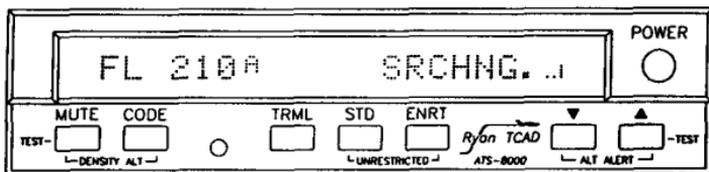
In the clear at FL 208, the Altitude Alert sounds and the aircraft is leveled at FL 210. ATC requests and confirms your altitude as Flight Level 210.
