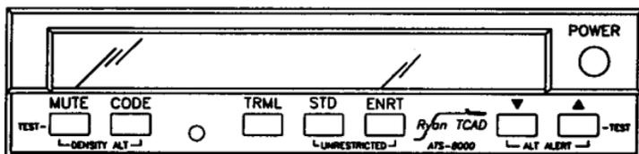
**POWER:** This is a push-on, push-off button for supplying power to the unit.
