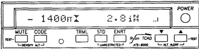
Passing through 10,000 feet, TCAD is placed in the ENRT mode, and a threat is indicated 1,400 feet below, closing in altitude at 2.8 iNM. Since the threat is closing in altitude, it is also climbing. Continue to monitor. You may want to visually acquire the traffic (see Scanning, Section IX, and Appendix 2).
