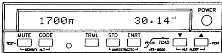
In the illustration above, current altimeter is 30.14" and the field elevation is 1700 feet MSL. If field elevation is not properly displayed, the altitude encoder is not supplying correct information, and may need additional warm-up time. After a few seconds, TCAD will enter a collision avoidance configuration (Search or Threat Acquisition).
