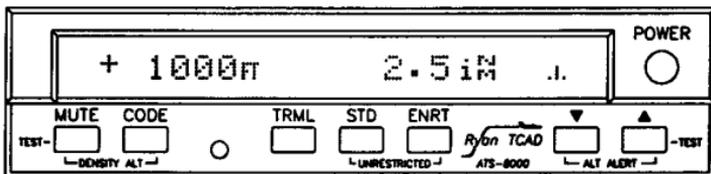
Traffic is acquired 1,000 feet above at 2.5 iNM. No tone is sounded because the traffic is outside the 2.0 iNM shield, even though it is displayed. No closure is indicated, therefore it is most likely not an imminent threat. Continue to monitor the traffic if desired.
