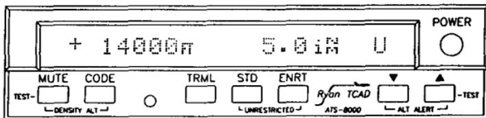
To monitor aircraft well beyond the shield, the Unrestricted Mode is selected (see Section III). Traffic is displayed 14,000 feet above and 5.0 iNM. A jet contrail is observed. Press code for the Mode A squawk and altitude.
