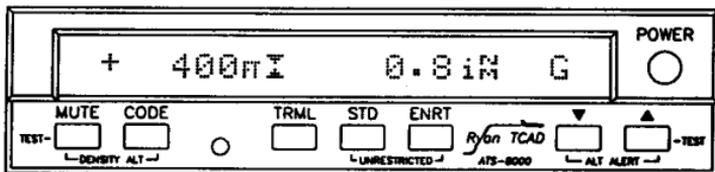
Before takeoff, check the area visually for traffic and check the TCAD. TCAD is indicating traffic 400 feet above, closing in altitude, and 0.8 iNM away. The traffic is then visually acquired on a close in base to final, and lands before your departure. Note the "G" on the right indicating Ground Mode.
