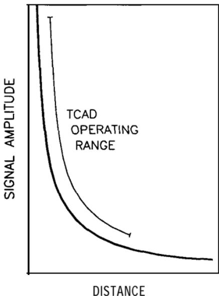
The range of a threat aircraft is determined from the arrival amplitude of the digital transponder signal. The amplitude of the signal is independent of code assignment. Amplitude changes with distance, and is used to calculate range and trend data. (See illustration to the left).
