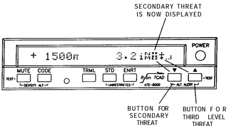
The secondary and third level threats can be displayed by pressing the ▼ or ▲ button appropriate to the threat. The secondary threat is displayed when the ▼ button is depressed. A third threat is displayed when the ▲ button is depressed.
