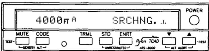
After leaving the airport area, select STD. At 3,800 feet, the Altitude Alert sounds indicating the aircraft is nearing 4,000 feet. The Built-in Test can be operated at any time (see Section X).
