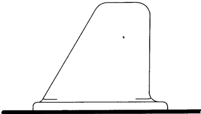
The TCAD antenna is an aerodynamically designed blade antenna normally mounted on top of the aircraft. The above illustration is one-half actual size.
