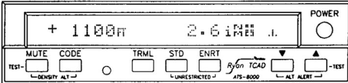
Pressing the ▼ button, corresponding to the secondary threat, shows additional traffic 1,100 feet above and 2.6 iNM. Note the airplane symbol is reversed (see Threat Acquisition, Section IV and Operating Tips, Section IX).
