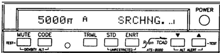
In the search configuration, a small upper case “A” appears on the display, indicating the Altitude Alert is engaged.
