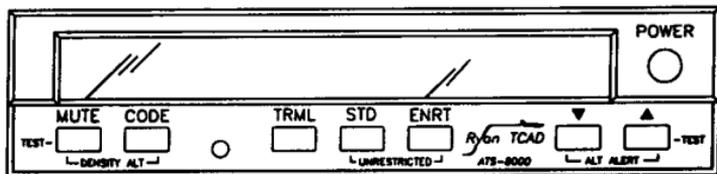
The Computer/Display unit is illustrated above at one-half actual size. This compact unit contains a high performance microwave receiver, an advanced high speed microprocessor based computer, and a bright character alphanumeric display. A Transponder Coupler is included to interface with the onboard transponder.
