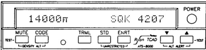
The code of the traffic is a secondary function, altitude and iNM are primary. In some situations, especially in high density areas, it may take a moment to acquire the code. If the code is not available, SQK: N/A will be displayed. The code of non-Mode C traffic is also available.
