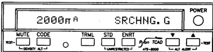
After climbing more than 200 feet, the "M" disappears, indicating that the alert tones are enabled. The mode symbol will indicate the Ground Mode until the aircraft climbs above the programmed base of the Terminal Mode (see Section III). Note the "A" remains, indicating that the Alert is set.
