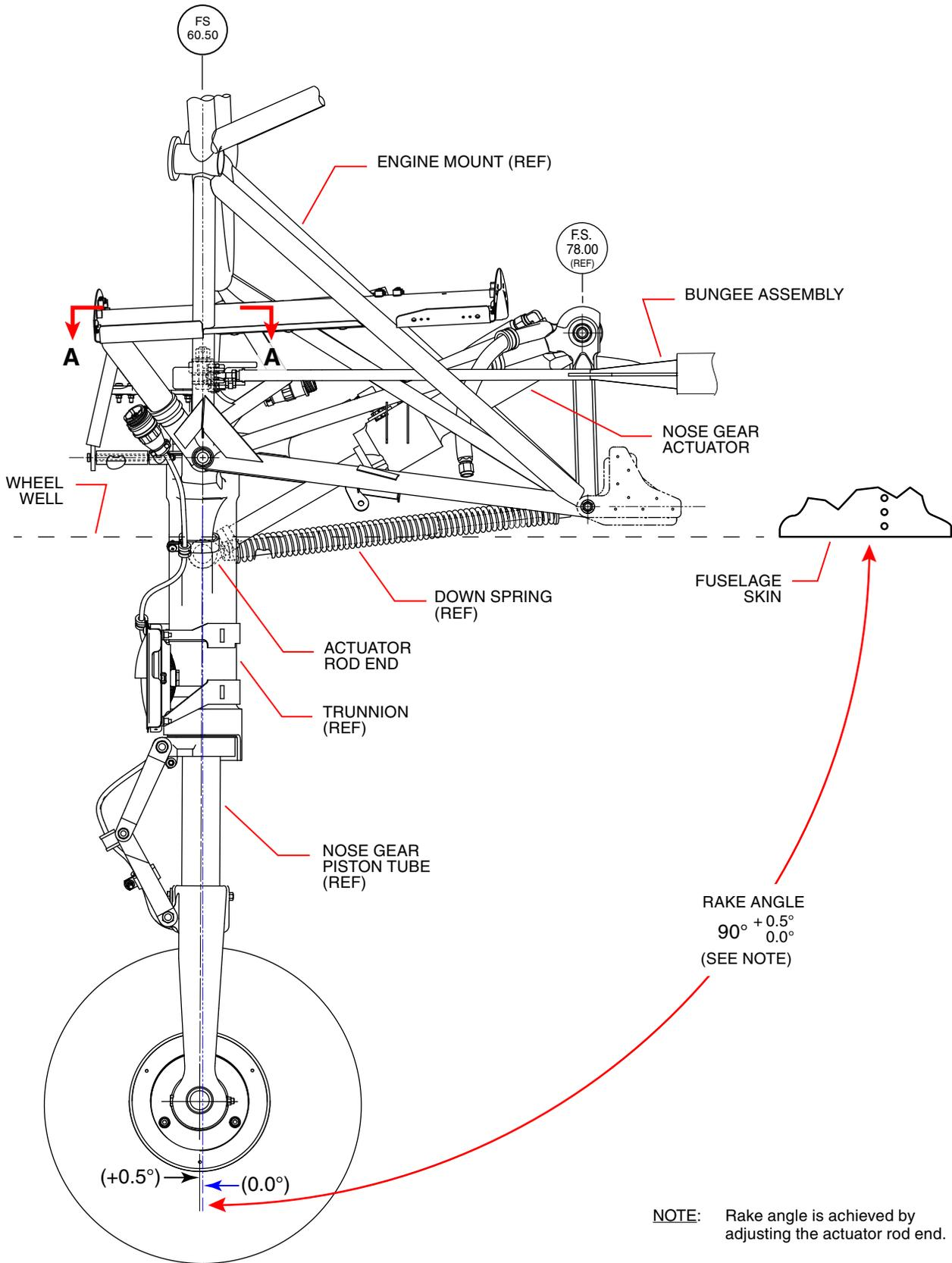
NOTE: Rake angle is achieved by adjusting the actuator rod end.
